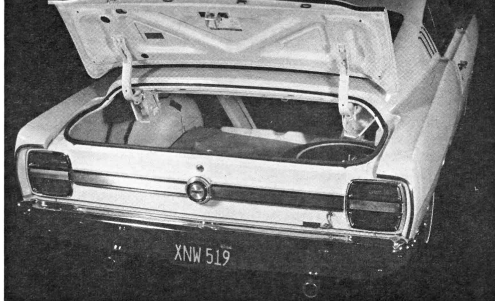
TRUNK SPACE is adequate, but limited. The sill is high, the trunk lid is small and most of the room is far forward. The spare tire rides in back, within easy reach.
